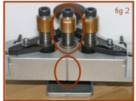
Place the jig on the edge of the door. The center groove (fig 2 ) on the jig should match upto the centre line you have just marked. Ensure the block buffers are tight against the door edge. Then clamp securely in the desired positions.
