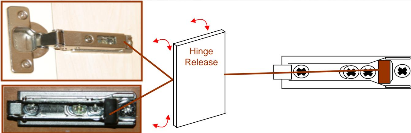
To release the hinge from the plate press the metal clip to the rear of the hinge plate.
