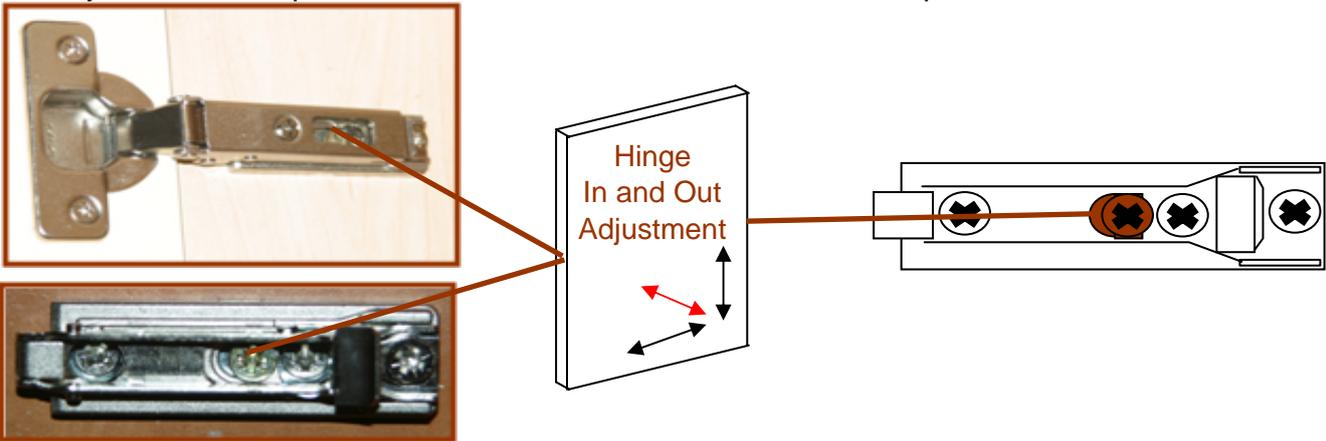
To Adjust the door in and out turn the screw in the centre of the hinge but located on the plate.
