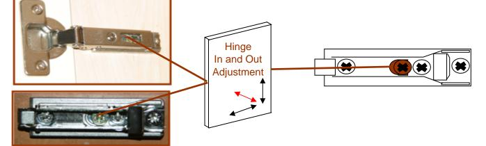
To Adjust the door in and out turn the screw in the centre of the hinge but located on the plate.
